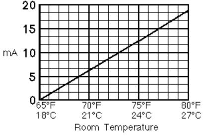
**Reverse Action** means that as the variable (for example, temperature) increases, the controller's output decreases. For example, as room temperature rises from 70 to 71°F, the controller output decreases from 8.1 to 7.3 mA. In the example below, as the sensor reads an increasing temperature, the controller responds by decreasing its output (pressure) to the valve, closing the normally closed valve and reducing the amount of heating.
