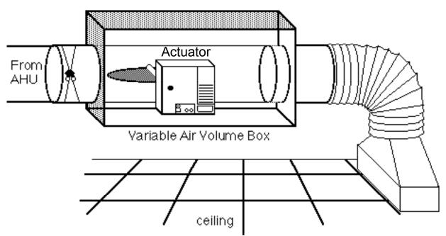
The VAV box has a **Damper** that modulates to maintain the space temperature by increasing or decreasing the volume of air being delivered to the space. The airflow is measured in <u>cubic feet per minute (CFM)</u> or *liters per second (L/s)*. If the space is too warm, the damper is adjusted to allow more 55°F (13°C) air into the space. If the space is too cool, less air is delivered to the space.
