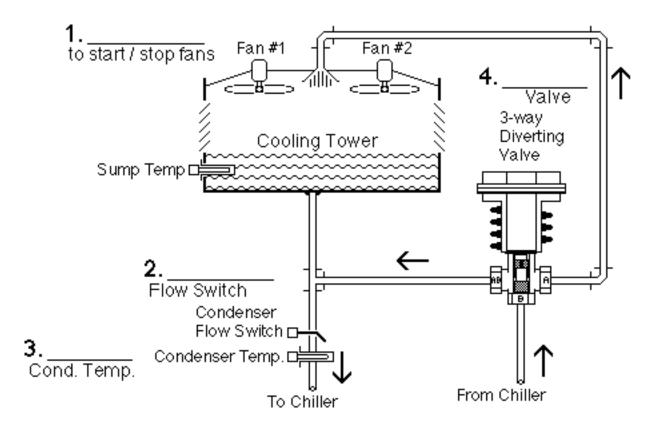
Identify the numbered points in the following diagram as either: AI, DI, AO, or DO
