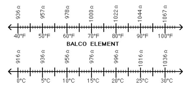
The resistance outputs of a Balco sensor follow the diagrams below:
