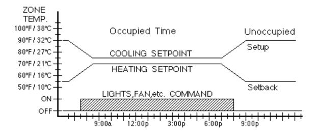
Time-Programmed Commands are an excellent way to save energy. However, this strategy is only effective if a building, or a large portion of a building, has an unoccupied time. During unoccupied time, typically at night, the heating setpoint shifts to 55°F (13°C) (*night setback*); the cooling setpoint shifts to 90°F (32°C) (*night setup*); and lights, fans, chillers, and other mechanical equipment are turned OFF.
