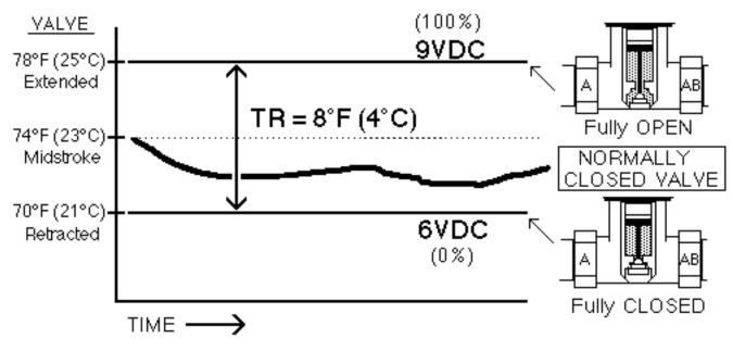
Throttling range is sometimes referred to as "sensitivity". Typical throttling ranges are 8° to 10°F (4° to 5°C) for mechanical controls such as mixed air control and the control of hot water supply. In contrast, room controls must be much tighter, with a throttling range between 2° and 4°F (1° to 2°C)
