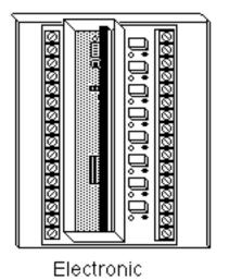
Many controllers are housed inside a control panel. In the case of the DDC electronic controls, the controller itself may be the control panel.
