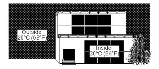
During the cooling season, if the inside temperature is considerably greater than the outside air temperature, then the air handling units may be turned ON during the night, to purge the warm air out of the building. This is called a Night Purge Cycle.
