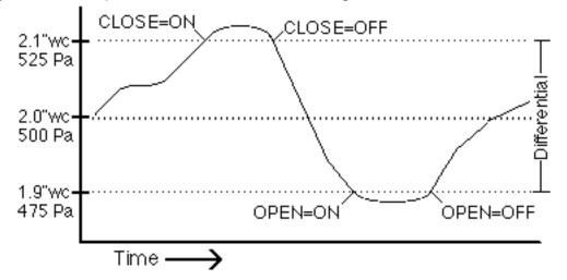
The diagram of static pressure controlled with floating control, is shown below.
