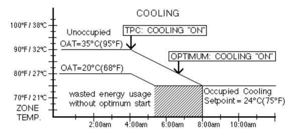
**Optimum Start** can be a valuable strategy for saving energy if there are unoccupied times in a building. The optimum start program computes the best, or optimum, time to start the heating or cooling equipment so that at the precise beginning of occupied time, the zone is at the desired temperature. Significant amounts of energy may be saved if the occupied setpoint is achieved as close to occupied time as possible.
