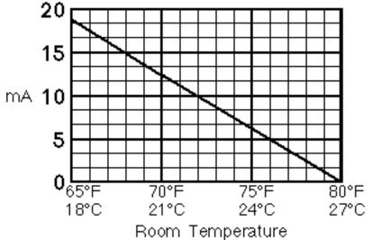
The action of the controller must match the proper HVAC application. Normally open heating valves always use direct acting controllers. If a reverse acting controller were to be placed on a normally open heating valve, the heating valve would open as temperature rises. A reverse acting controller never properly controls a normally open heating valve.
