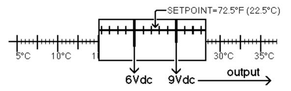
A signal from the sensor is sent to the controller. In this example,  $72.5^{\circ}F$  ( $22.5^{\circ}C$ ) is the setpoint or desired temperature for a room.
