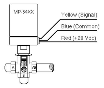
*Hydraulic actuators* and valve assemblies are another type of controlled device. The actuator in the diagram above operates on 6 to 9 Vdc. The yellow wire is the signal provided by a controller, and the blue wire is common, or 0 Vdc. The red wire is a source of +20 Vdc used by certain controllers but is typically not a power supply to DDC control systems controllers. Hydraulic actuators use hydraulic fluid to extend the shaft of the actuator. An internal spring is used to retract the actuator.
