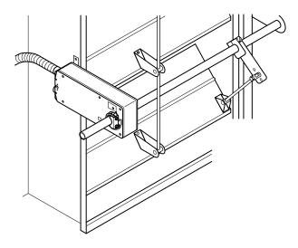
When used on dampers, direct-coupled DuraDrive<sup>™</sup> actuators require minimal or no external linkage, making installation easy to perform. DuraDrive actuators may also be used with ball and globe valves, and are also available as complete actuator and valve assemblies. They are manufactured in a variety of models, including <u>spring-return</u>, non-spring return, two-position, proportional, and floating control.
