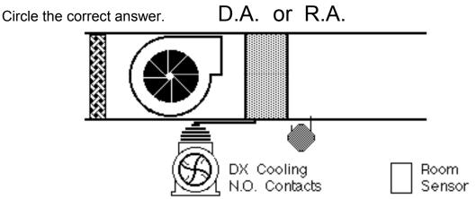
5. The mixed air sensor modulates the normally closed outside air dampers and the normally open return air dampers to maintain a temperature of 55°F (13°C). What action is needed for the controller?
