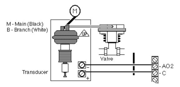
Another E-P transducer converts a 4 to 20 mA current signal to a 3 to 15 psig pneumatic signal. Setup is required on this transducer also, to adjust the current signal to the desired pneumatic output signal.
