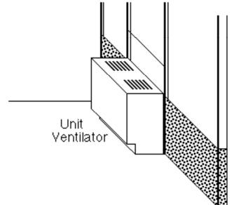
A **Unit Ventilator**, common in schools, is shown above. It serves as the local airhandling unit and has dampers for the outside and return air, a fan, and a hot water coil. The hot water comes from the boiler. The diffusers are on the top of the unit. A space thermostat controls the valve and dampers in this unit. A switch on the base of the thermostat starts the fan inside the unit ventilator.
